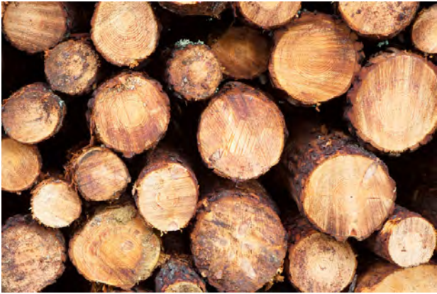
Diagram 8.3—Green Wood Logs: no checking visible, indicates green, freshly cut wood.
