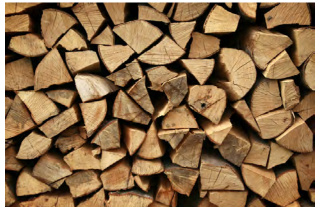
Diagram 8.2–Seasoned, Split Wood: checking visible, indicates wood has been seasoned.
