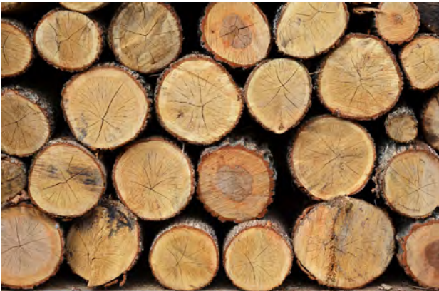
Diagram 8.4—Seasoned Wood Logs: checking visible, indicates wood has been seasoned.
