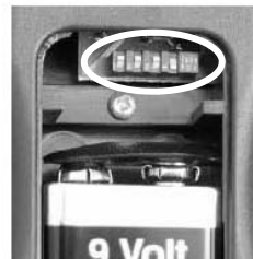
DIP Switch in Remote Handset Battery Compartment
