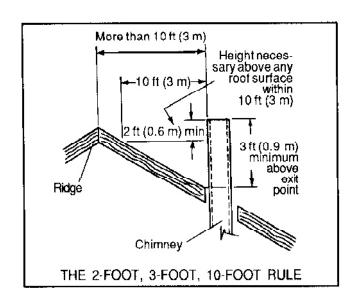
Codes require that solid-fuel chimneys extend 3 ft (0.9 m) above the point at which they exit from the roof, provided that no part of any structure is within the top of the chimney, then the chimney must extend 2 ft (6 m) above the highest point with the 10 ft (3 m) radius top height. If there is not ten feet of clearance from the top of the chimney, then the chimney must extend 2 ft (6m) above the highest point with the 10 ft (3m) radius.
