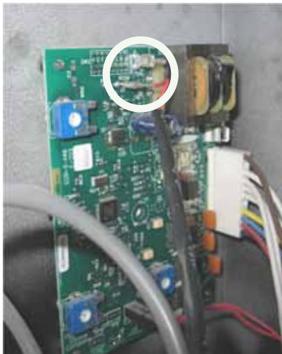
The optional Room Sensor cable attaches to two bare terminals on the rear of the circuit board. These connections are not polarity specific.
