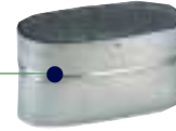
Stainless Steel Dripless Type "A" Oval Connector Part # 2CNNTRA ___Dia. Available in 6", 7", 8", 10" Diameters Used to join Z-FLEX Oval Liner to Oval T-Section and Oval to Oval Liner or when going through a fireplace adapter.
