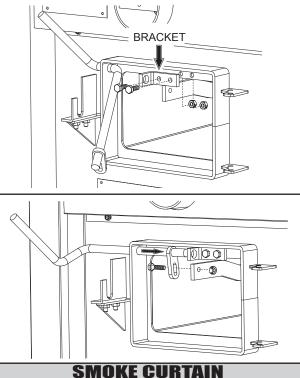
Using two  $1/4-20 \ge 1-1/4''$  Carriage bolts, the smoke curtain clips and two nuts, attach the smoke curtain in place above the Fuel Feed Door as shown below. After installation, the smoke curtain should swing freely back into the furnace.
