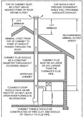
1. The furnace should be the only heating using the chimney flue One furnace per flue outlet.
