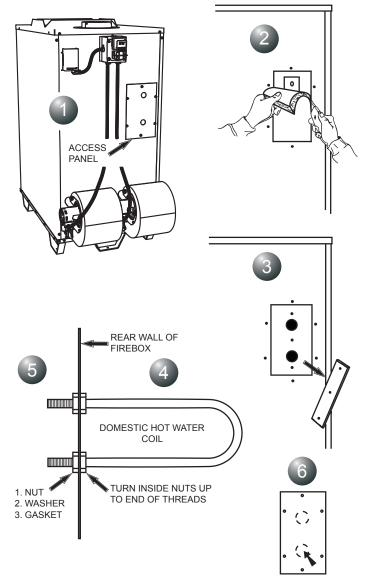
This Furnace will accept the installation of a Domestic Hot Water Coil Kit. The U.S. Stove kit is a 1124 Water Coil and it may be purchased from your local dealer.
