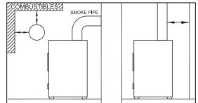
According to NFPA standards, single wall stove pipes can be within 9" of combustibles provided an approved fire retardant material covered with 28 gauge sheet metal, spaced out 1" on non-combustible spacers, is utilized. See illustration.
