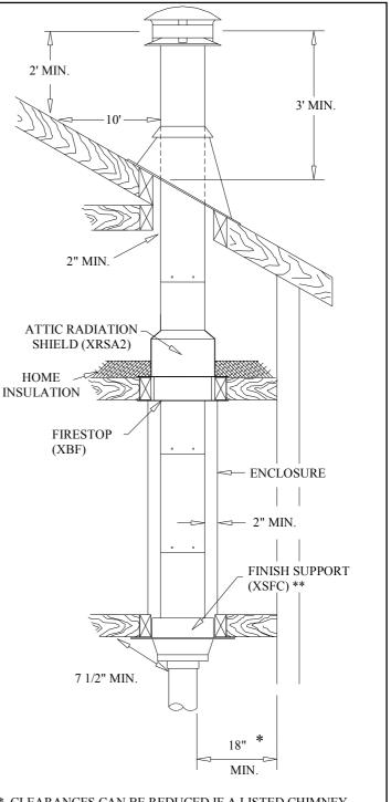
\* CLEARANCES CAN BE REDUCED IF A LISTED CHIMNEY CONECTOR IS USED INSTEAD OF A SINGLE WALL CONNECTOR
