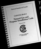
The use of plastic venting systems on gas fired water heaters, furnaces and boilers is undergoing a significant change. In the summer of 2006 the CSA B149.1 Natural Gas and Propane Installation Code was amended to require all plastic venting materials to be certified to ULC S636. The code change is effective January 1, 2007.
