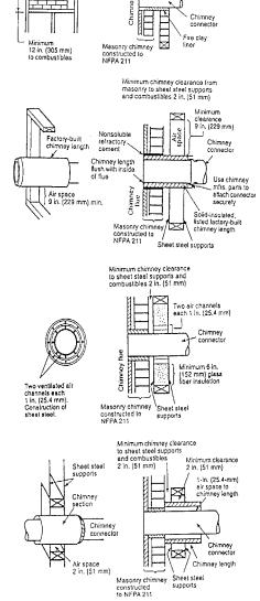
Minimum chimney clearance to brick and combustibles 2 in, (51 mm)
