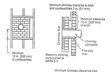
masonry to sheet steel supports and combustibles 2 in, (51 mm) Minimum clearance Nonsoluble Factory-built
