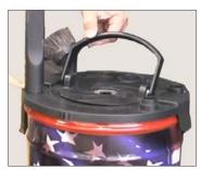
Keep BOBCAT lid on canister while cleaning filter. Lift and release the instant filter cleaning handle 5 times.
