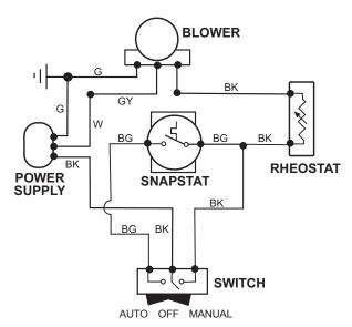
Figure 22. Blower Wiring diagram.
