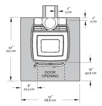
Figure 9. Floor Protection minimum dimensions, U.S.
