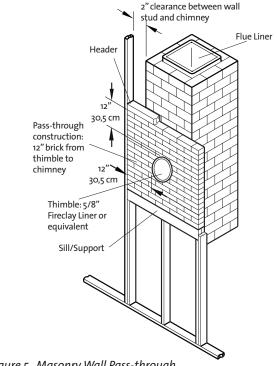
Figure 5. Masonry Wall Pass-through.
