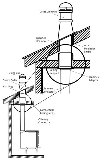
Figure 8. Prefabricated Listed Type HT Chimney.
