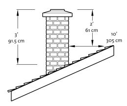
Figure 4. Chimney Height Requirement.
