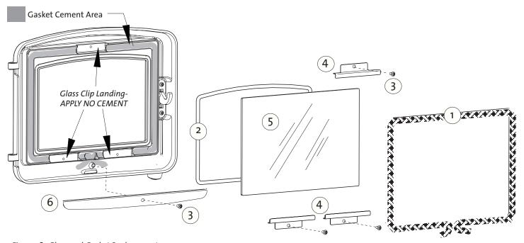
Figure 18. Glass and Gasket Replacement
