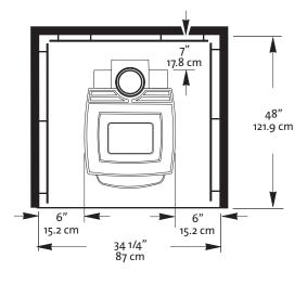
Figure 12. Alcove with Wall Protection.
