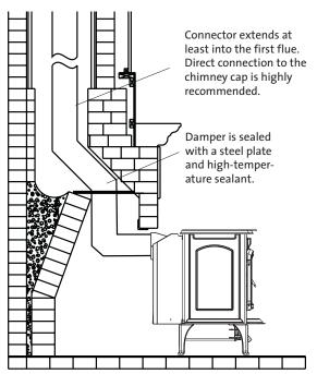
Figure 7. Hearthmount Installation.
