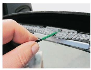
Figure 19. Loosen the glass clips.
