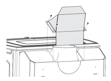
Figure 2. Flue Collar heat shield attachment.
