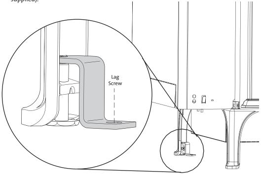
Figure 25. Floor Bracket Detail
