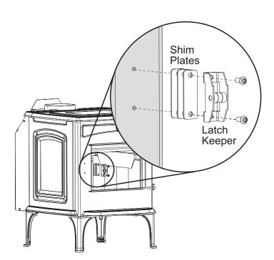
Figure 17. Latch adjustment.
