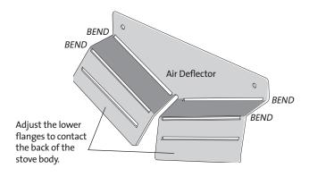
Figure 19. Air Deflector orientation.
