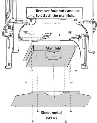
Figure 23. Outside Air Adaptor installation.
