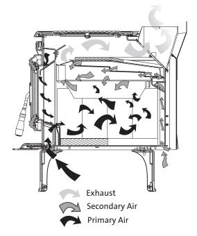
Figure 15. Combustion air paths
