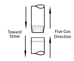
Figure 3. Chimney connector orientation.
