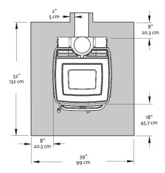
Figure 10. Floor Protection minimum dimensions, Canada.
