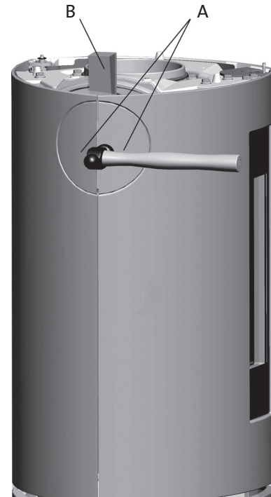
Figure 10. Removing the rear exit outlet knock-outs.
