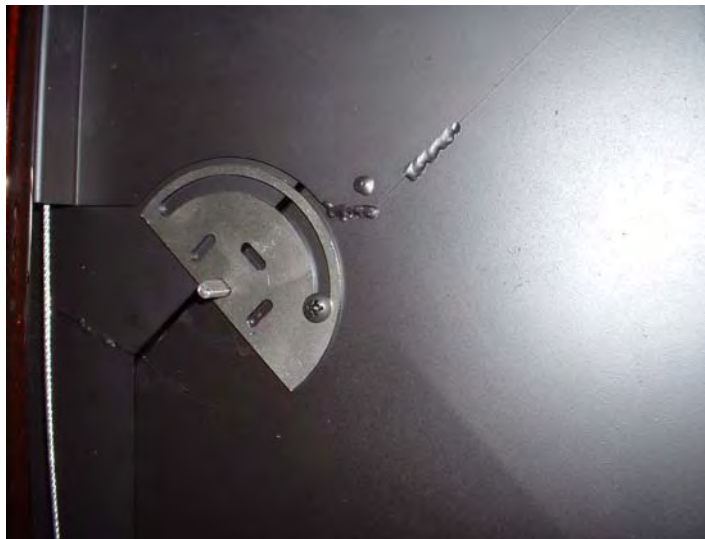
Photo 13: Restrictor Fully Closed
