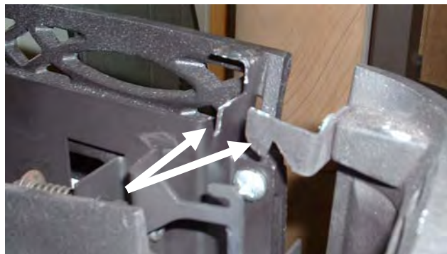
Photo 9 – Front Panel Mounting Tang Detail
