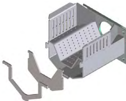
This figure shows the new end gate which gets installed without the stirring rod.
