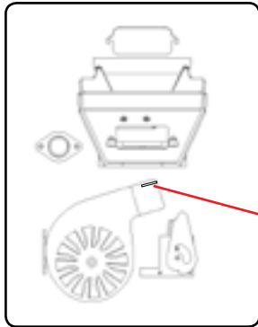
Fig. 30 Exposed blower wheel and flue opening, NOTE: ESP probe is visible.
