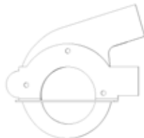
Blower cover removed.
