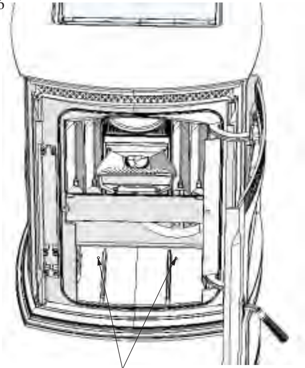
Unit bolt down holes for mobile home installation lag to floor with 1/4" lag bolts with washer (supplied by installer.)
