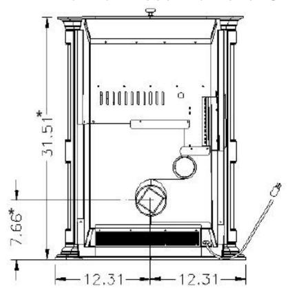
\* Note: Installation of the optional leg kit adds 2.95 inches of height.
